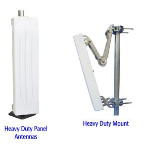
The Panel Antenna series contains four different models, ranging from 13 dBi to 17 dBi gain and covering the entire WiMAX band at 2.5-2.7 GHz. The corresponding beamwidths for these antennas range from 45° to 120° sectors.
